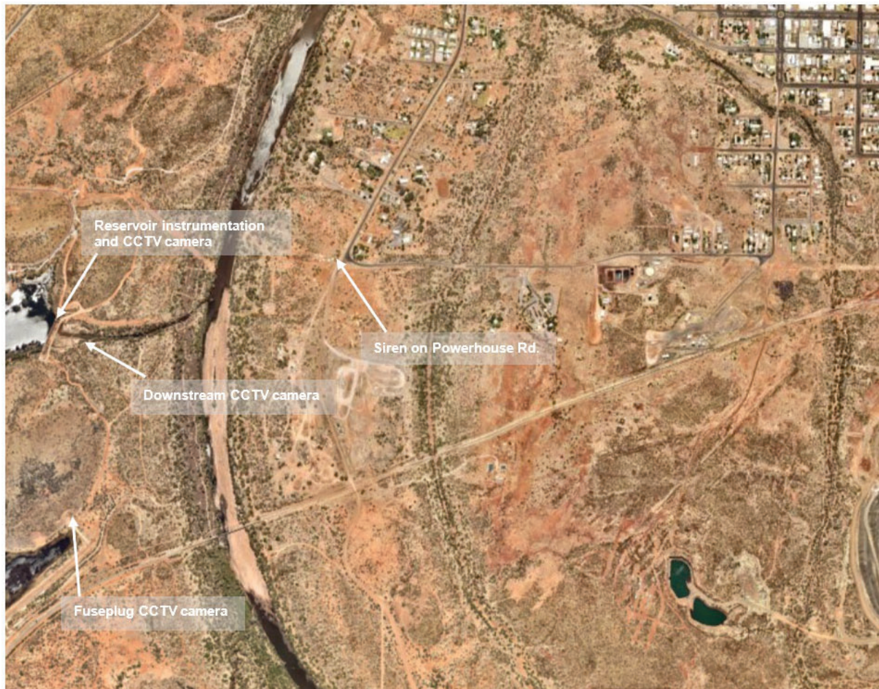
Figure 5 Scada Instrumentation Plan (Nearmap, 2024)
